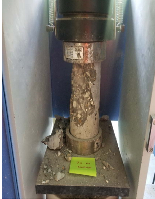
Figure 45. 72- Hour Compressive Strength Specimen
