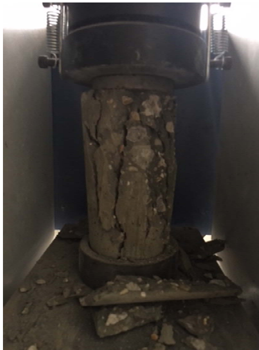
Figure 14. Failure of mixtures with RAC and 20 oz AC.
