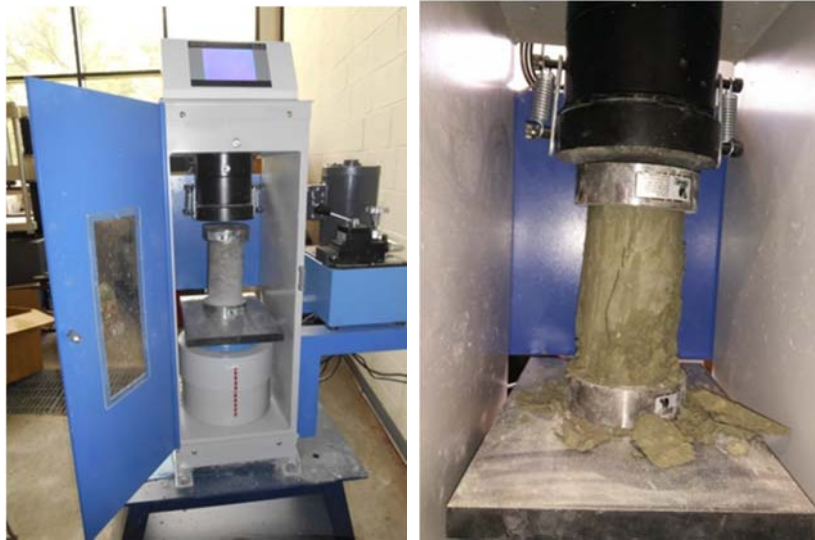
Figure 6. Compression Tester and 4-hour Compression Test
