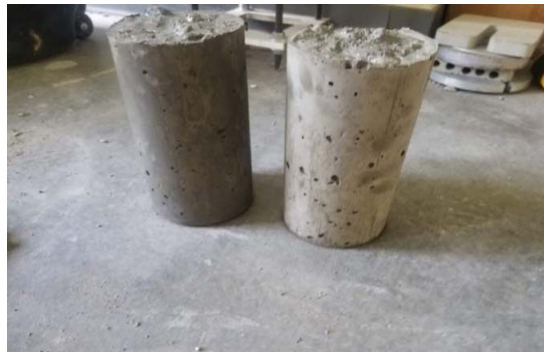
Figure 37. 10 lbs. of Water Mixture Specimen
