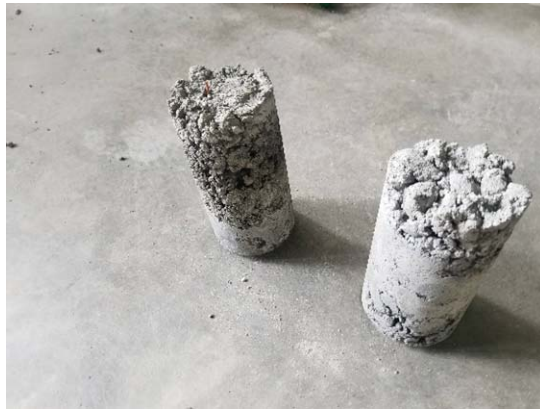
Figure 36. 9.5 lbs of Water Mixture Specimen
