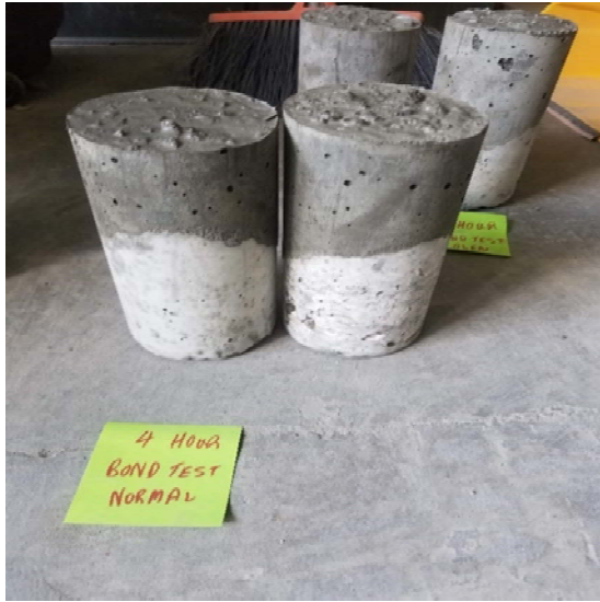
(a) Before Test (b) After Test Figure 39. 4 Hour Bond Strength Test Specimen
