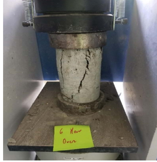
(a) Air-Dry Specimen (b) Oven Dry Specimen Figure 40. Specimens Tested after 6 Hour Curing
