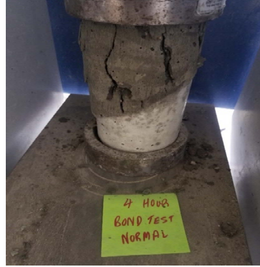
(a) Before Test (b) After Test Figure 39. 4 Hour Bond Strength Test Specimen
