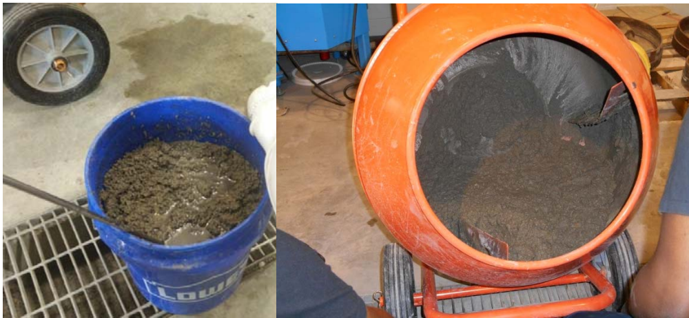
Figure 5. 24-hour Soaked LWA for Concrete Mix
