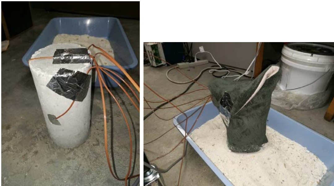
Figure 20. Temperature Measurement Inside of the Blanket with Thermocouples
